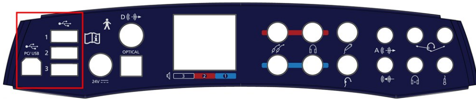
Fig. 2 Connectors isolated from patient transducers - AURICAL Aud connection panel
